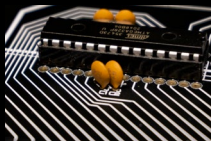
ATmega328P's Decoupling Capacitors
